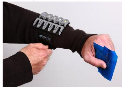
The *Chameleon*<sup>®</sup> Chemical Suicide Detection Kit contains sensors for: high pH (base), hydrogen sulfide, low pH (acid), phosphine, and sulfur dioxide. For more information on any of the *Chameleon*<sup>®</sup> Detection Kits visit [www.morphotec.com](http://www.morphotec.com).
